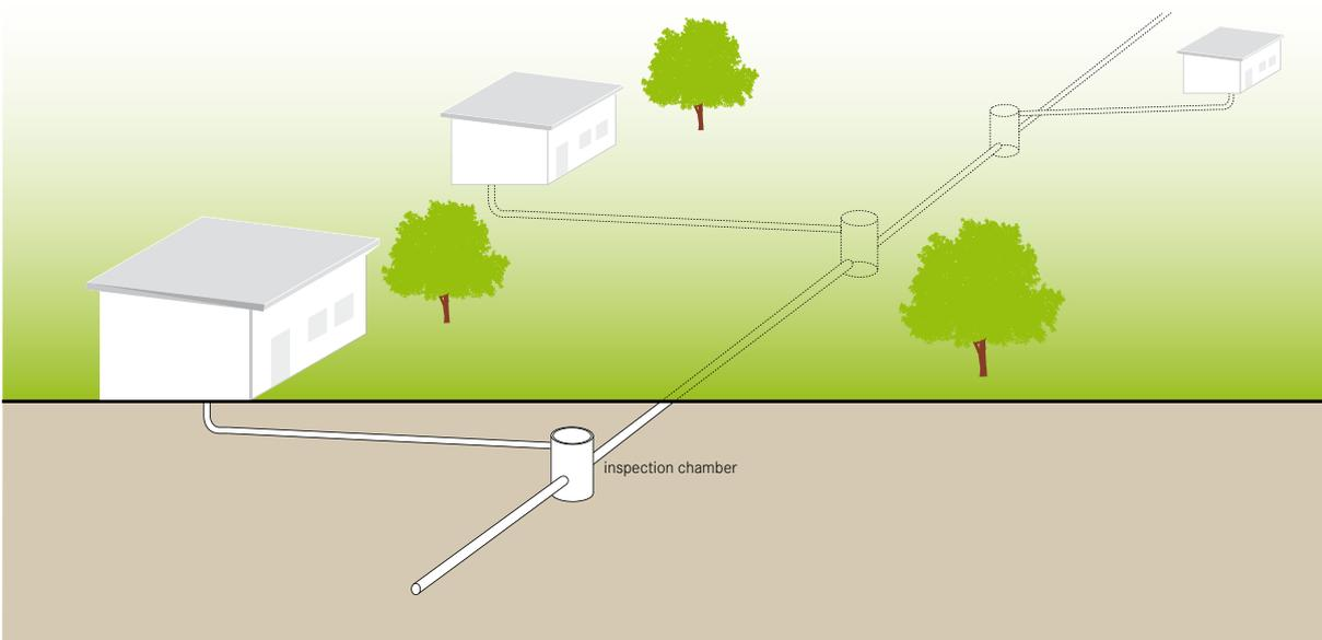
**A simplified sewer describes a sewerage network that is constructed using smaller diameter pipes laid at a shallower depth and at a flatter gradient than Conventional Sewers (C.6). The simplified sewer allows for a more flexible design at lower costs.**
